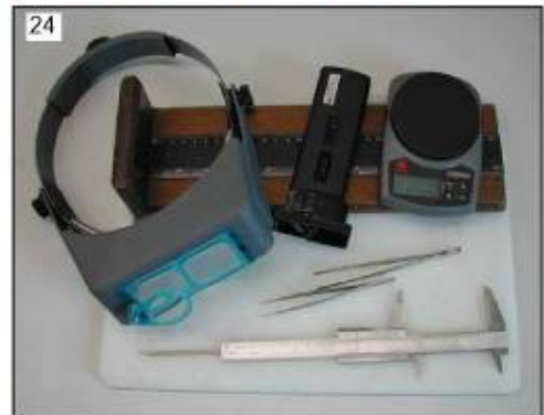
Plates 19-24 (19-22) Electrical fishing with a Smith-Root LR-24 backpack electrical fishing unit, (23) recording site data on the middle reaches of the Kells Blackwater, (24) equipment used to examine larval lampreys; headband magnifier, measuring board, handheld balance, calipers, tweezers, white board, and portable microscope.
